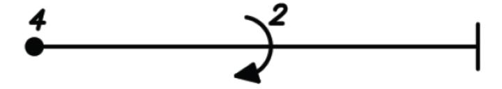
**Two Point Roll (K=3):** The model starts in straight and level flight and before centre rolls at a uniform rate through 180 degrees to inverted then pauses ('for a heart beat'), then rolls another 180 degrees in the same direction to finish in upright flight. The model should pass through centre inverted. The approximate time of the manoeuvre is three seconds.
